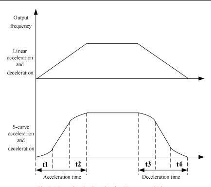
Fig. 7-16 Acceleration/Deceleration Time Control Diagram
