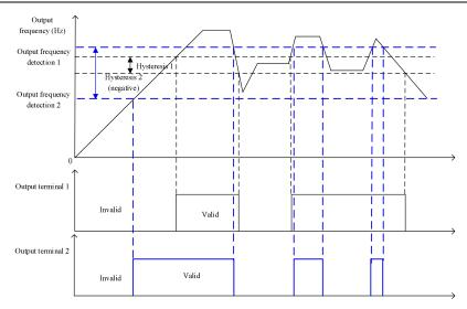
Fig. 7-37 Schematic Diagram of FDT Detection
