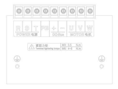
d) Schematic Diagram of Terminals (EM730-030-3/3B~EM730-037-3/3B)
