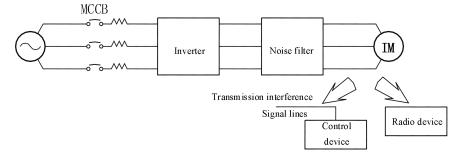
Fig.3-7 Noise Filter Installation on Output Side
