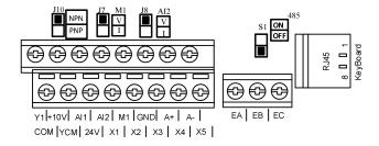
Fig.3-11 Layout of Control Circuit Terminals 1
