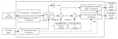
Fig. 7-42 Block Diagram of Counting Function
