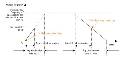
Fig. 7-32 Schematic Diagram of Jog Running
