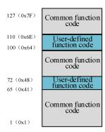
Fig. 12-21 Classification of MODBUS Function Codes
