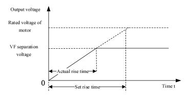
Fig. 7-20 Rise Time Description of VF Separation Voltage
