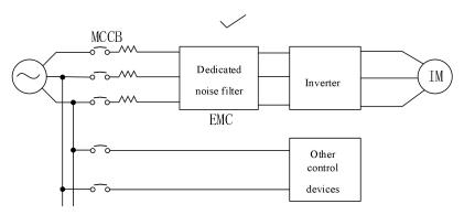
Fig.3-5 Correct Installation of Noise Filter
