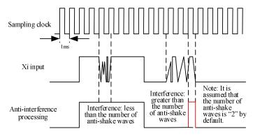
Fig. 7-13 Schematic Diagram of Terminal Filter Sampling
