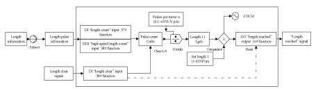
Fig. 7-40 Block Diagram of Fixed-length Counting
