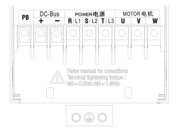
b) Schematic Diagram of Terminals (EM730-2R2-3B~EM730-4R0-3B)
