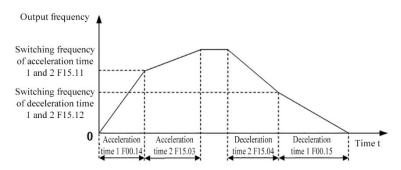
Fig. 7-34 Schematic Diagram of Automatic Switching of Acceleration and Deceleration Time During acceleration, if the output frequency is less than the switching frequency of the
