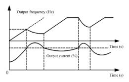
Fig. 7-25 Current Limit Process
