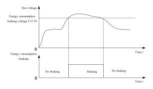
Fig. 7-39 Schematic Diagram of Energy Consumption Braking
