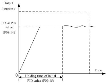
Fig. 9-29 Schematic Diagram of Initial PID Output
