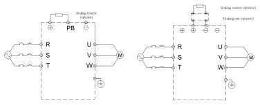
Fig.3-3 Standard Wiring of Main Circuit
