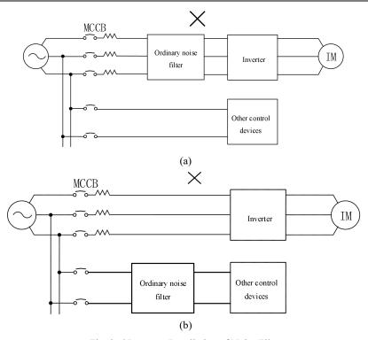
Fig. 3-6 Incorrect Installation of Noise Filter
