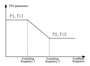
Fig. 7-21 Schematic Diagram of PI Parameters
