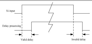
Fig. 7-14 Schematic Diagram of Terminal Delay Sampling
