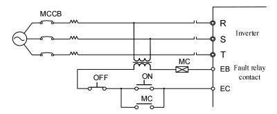
Fig.3-4 Connection of Input Circuit Breaker
