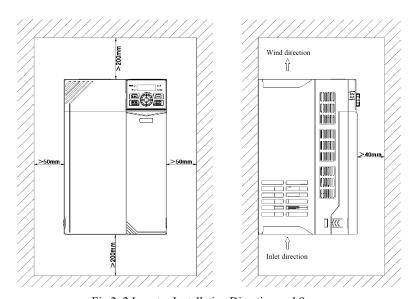
Fig.2-2 Inverter Installation Direction and Space
