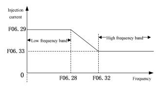
Fig. 7-22 Schematic Diagram of High Frequency Injection
