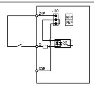
a: Use of internal power supply in NPN mode
