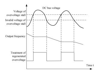
Fig. 7-23 Schematic Diagram of Overvoltage Stall Protection
