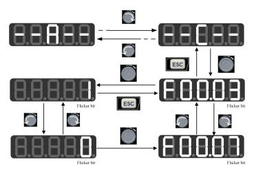
Fig. 4-5 Function Code Modification in Non-default Mode
