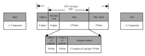
Fig. 12-20 Schematic Diagram of Message Frame in RTU Mode
