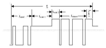
Fig. 4-23 Timing Parse Diagram of Complete Data Frame
