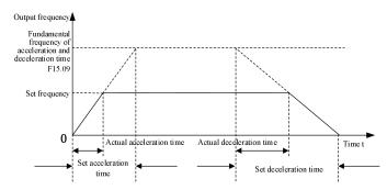
Fig. 7-33 Schematic Diagram of Acceleration and Deceleration Time
