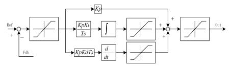
Fig. 7-27 Block Diagram of Process PID
