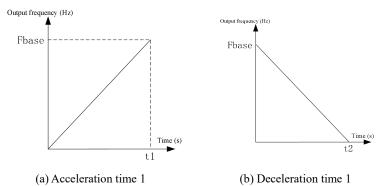
Fig. 7-9 Acceleration and Deceleration Time
