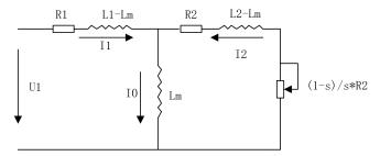
Fig. 8-18 Equivalent Circuit of Three-phase Asynchronous Motor
