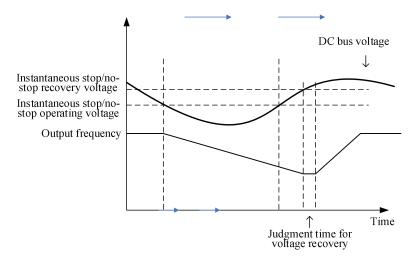
Fig. 7-24 Schematic Diagram of Instantaneous Stop/Non-stop Deceleration Function
