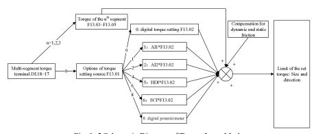
Fig. 1-5 Schematic Diagram of Torque Input Mode
