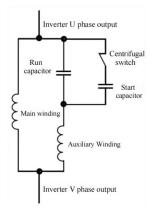
② Remove the running capacitor: connect the inverter U phase to one end of the main winding, the V phase to one end of the auxiliary winding, and short-circuit the other ends of the main and auxiliary windings together and connect them to the inverter W phase.
