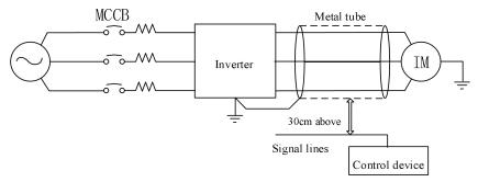
Fig.3-8 Solution to Inductive Interference
