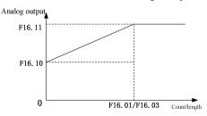
Fig. 7-17 Schematic Diagram of Analog Output of Count and Length
