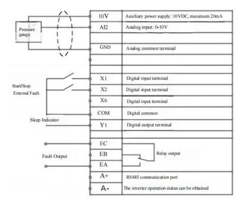
Wiring corresponding to application macro F16.00=1 (remote pressure gauge voltage feedback mode)
