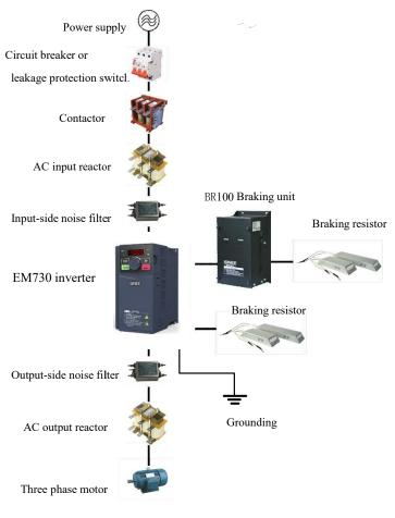
Fig.3-1 Connection of Inverter and Peripheral Devices
