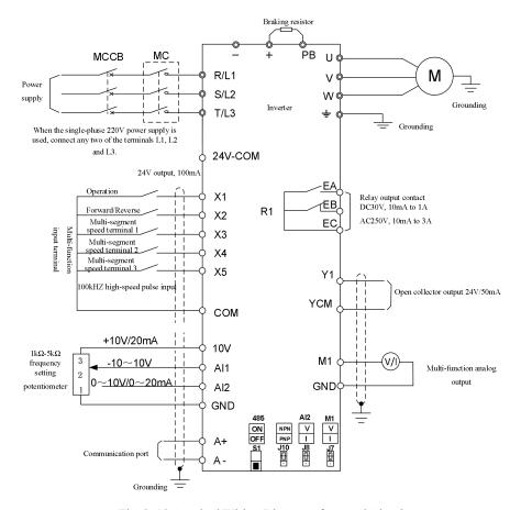
Fig. 3-19 Standard Wiring Diagram of Control Circuit
