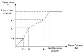
Fig. 7-19 Schematic Diagram of Multi-point Polyline V/F Curve
