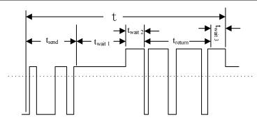
Fig. 7-31 Timing Parse Diagram of Complete Data Frame
