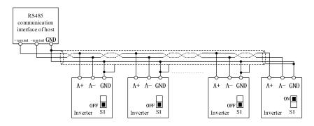
Fig. 3-17 Wiring of Communication Terminals of Multiple Inverters
