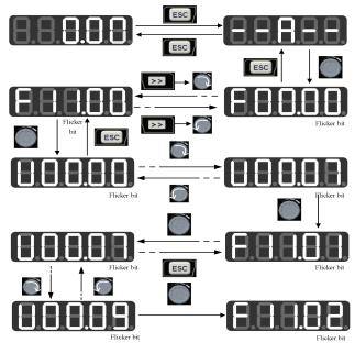
Fig. 4-4 Example of User-defined Mode Setting
