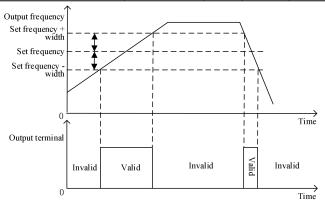
Fig. 7-36 Schematic Diagram of FAR Detection
