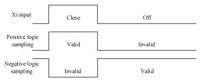
Fig. 7-12 Schematic Diagram of Positive/Negative Logic Sampling of Terminal
