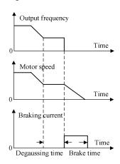
Fig. 7-17 DC Braking Process for Start
